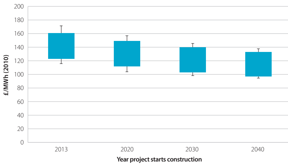
Figure 10: Levelised cost of new dedicated biomass, high-low discount rate range (2011-2040)
